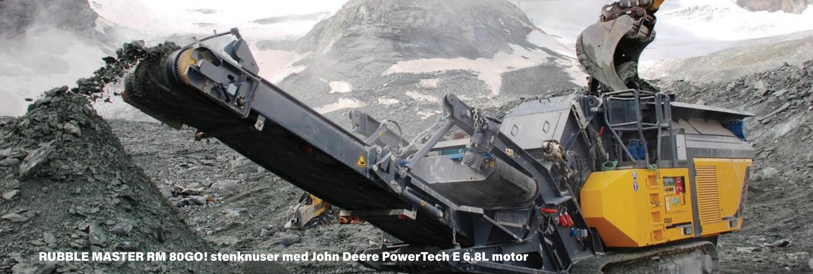
**RUBBLE MASTER RM 80GO! stenknuser med John Deere PowerTech E 6.8L motor**
